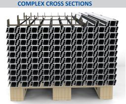
The **FLEXICOMB** can be used in many different ways. Some profiles and parts can be very difficult to pack depending on its cross section. The comb is flexible and can be angeled during packing and sometimes you can pack two parts in the same "rack".
