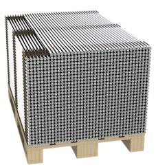
The **FLEXICOMB** gives you stable packages. Round items can be very difficult to pack on top of each other. The walls on each comb will support the next layer and enhance the stability during transport and storage.
